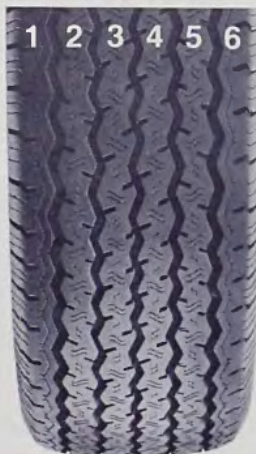
Sears RoadHandler, 13% wider tread. 10% deeper tread (at center). Extra tread row.
